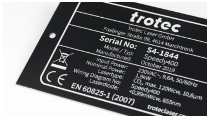
Laser engraving of data plates
